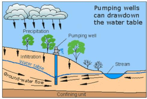
rate that it is replenished, either by infiltration from the surface of from streams, then the water table can become lower, resulting in a "cone of depression" around the well. Depending on geologic and hydrologic conditions of the aquifer, the impact on the level of the water table can be short-lived or last for decades, and it can fall a small amount or many hundreds of feet. Excessive pumping can lower the water table so much that the wells no longer supply water—they can "go dry."
