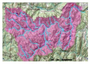
Figure 3. View of the StreamStats map frame showing an upstream network trace for a user-selected point on a stream in Massachusetts.
