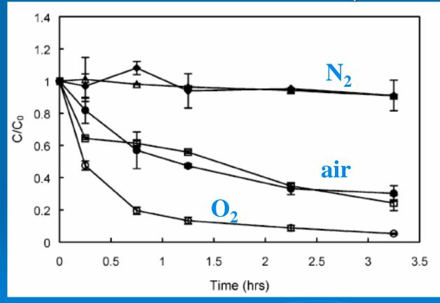
[molinate]=0.2 mg/L[nZVI] = 560 mg/L; pH 4
