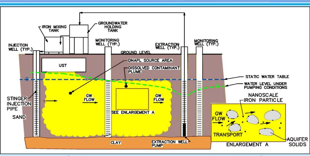
300 lb BNP (99.9 % Fe, 0.1 % Pd and polymer support) Gravity Feed, 10 injection points
