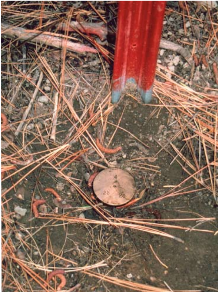
Figure 5—Grid point marker displaying the treatment unit number (4) and the UTM coordinates (25 24) in the Goosenest AMA.
