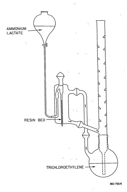
Fig. 3--Column apparatus for separations with lactate.
