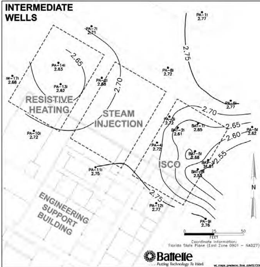
Figure 2-8. Pre-Demonstration Water Levels (as Elevations msl) in Intermediate Wells at Launch Complex 34 (September 1999)
