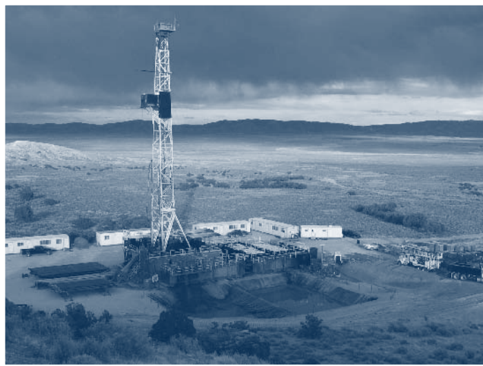
A drilling operation exploring for oil and gas at Pancake Summit northwest of Ely. Photo courtesy of: Plains Exploration and Production Co.
