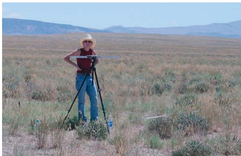
Figure. A Laser Point Bar projects points of light on the ground to generate data that can be used for measuring ground cover.
