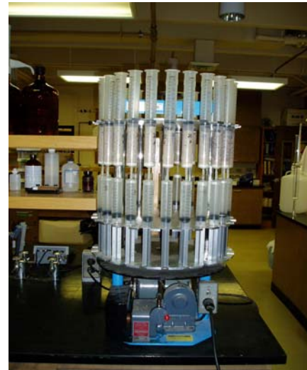
Figure 4. Column experiment setup used to evaluate the cation exchange kinetics between CBNG water and different sizes of St. Cloud zeolites.
