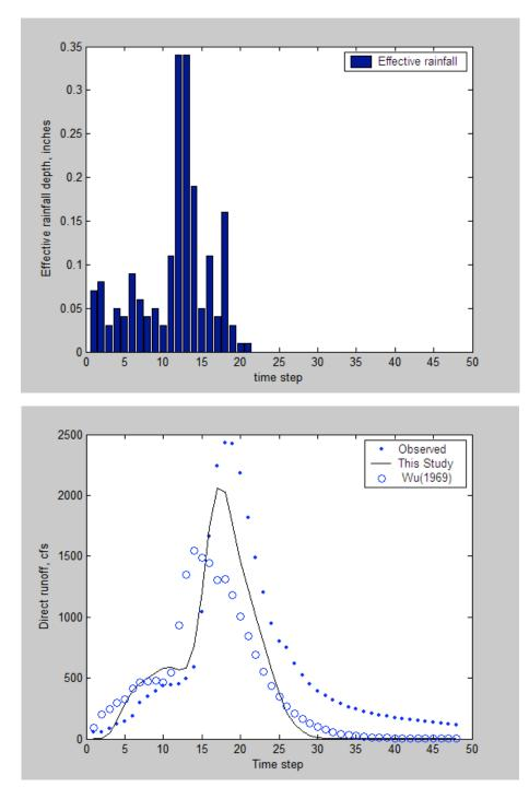
Figure 2. Prediction of storm runoff of Wahiawa Stream at USGS gaging station 10268000, October 29-30, 2005
