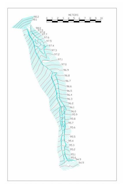
**Figure 3.** *Channel topography. Survey conducted in July 2006. Datum elevation is 100 m (arbitrary).*
