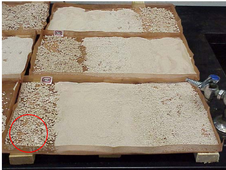
Figure 1. Photo of manufactured limestone-based granules. Granules in the red circle are about 1-2 mm in diameter.
