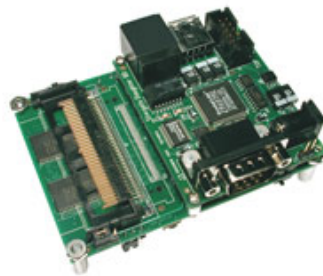
Figure 2: Stargate Gateway used to receive network data packets for database storage. This is known as the server/gateway node.
