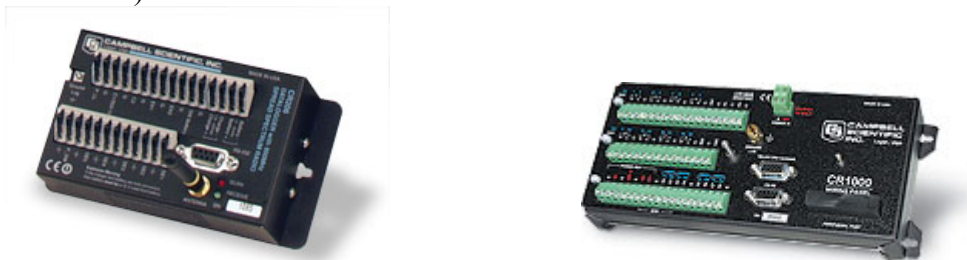
Figure 4: Campbell Scientific CR206 (left) and CR1000 (right).
