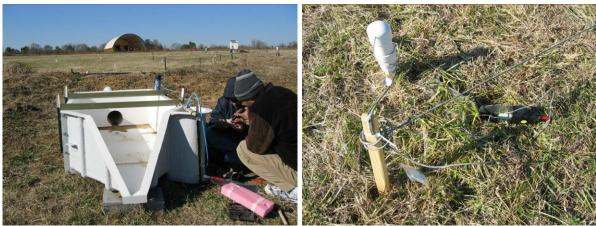
Figure 1. Instrumented hillslope with surface and subsurface sensors (detailed view on the right), H-flume, rain gage, and shallow wells at the Sand Mountain Research and Extension Center, Crossville, Dekalb County, Alabama.
