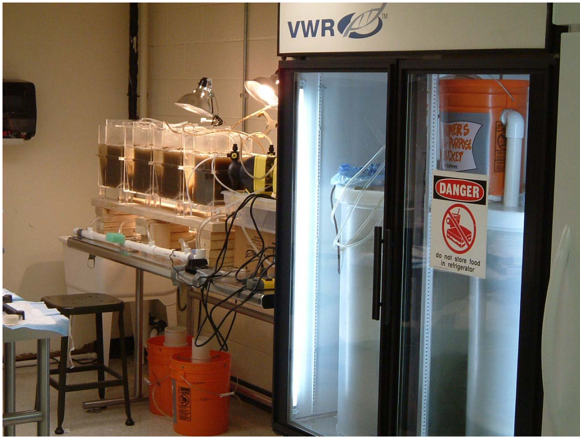
Figure 3. Bench-scale biological treatment process.
