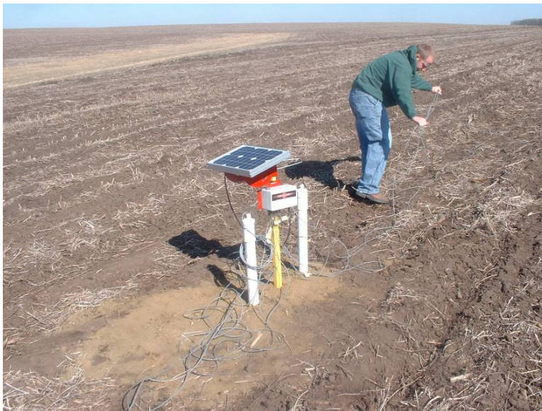
Figure 1. Ultrasonic sensors atop two piezometer tubes, wire to the control module, and solar panel. The additional wire leads to other sensors (not shown).
