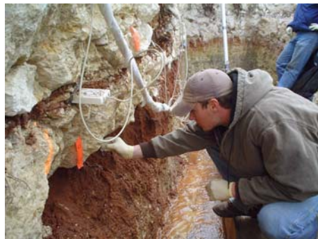
Figure 2. Water Sampling During a Dye Tracer Test at Honey Creek State Natural Area
