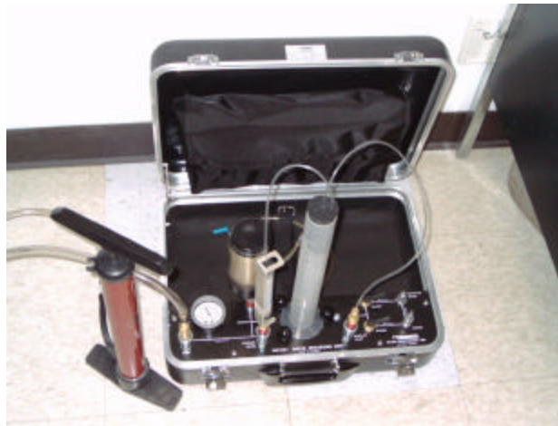
Water Degassing Unit
