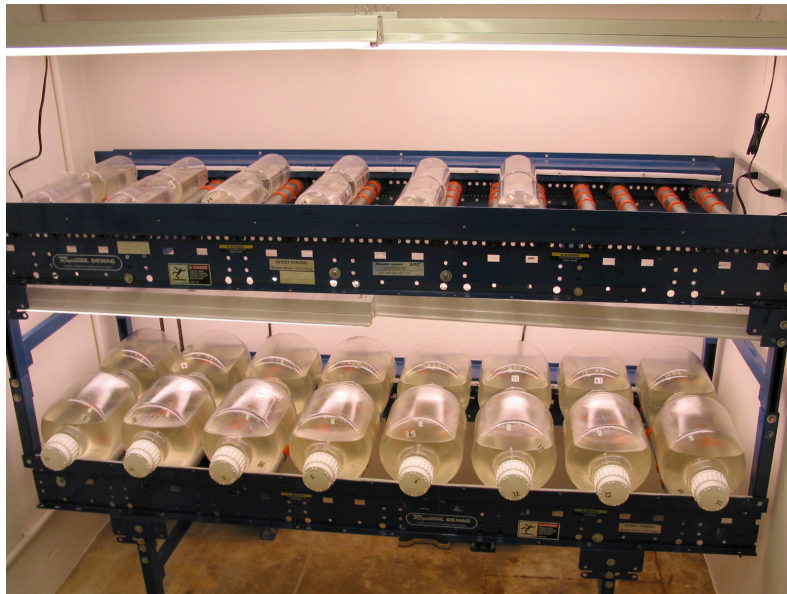
Figure 4. UOBS bottle roller, showing 16 macrozooplankton (12-L bottles; bottom) and 12 microzooplankton (2.5-L bottles; top) mesocosms. Bottles rotate at 1-4 revolutions per minute and change directions every 5 minutes to prevent sedimentation and aggregation of planktonic particles. Ambient temperature and light are maintained to mimic lake conditions of interest.
