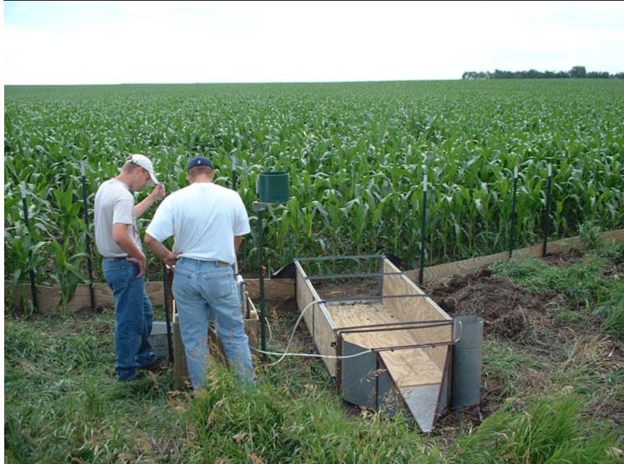
Figure 1 - Installation of sampling equipment on tile-only waterway.
