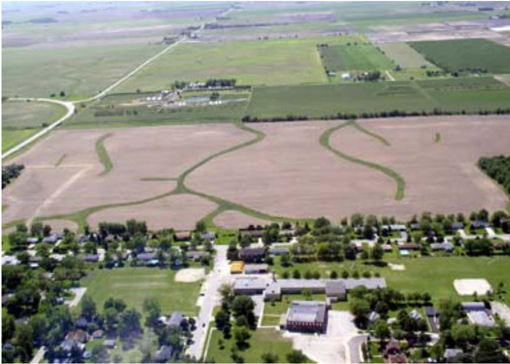
Figure 6.—Grassed waterways in agricultural areas help to remove excess surface water and prevent the formation of gullies.
