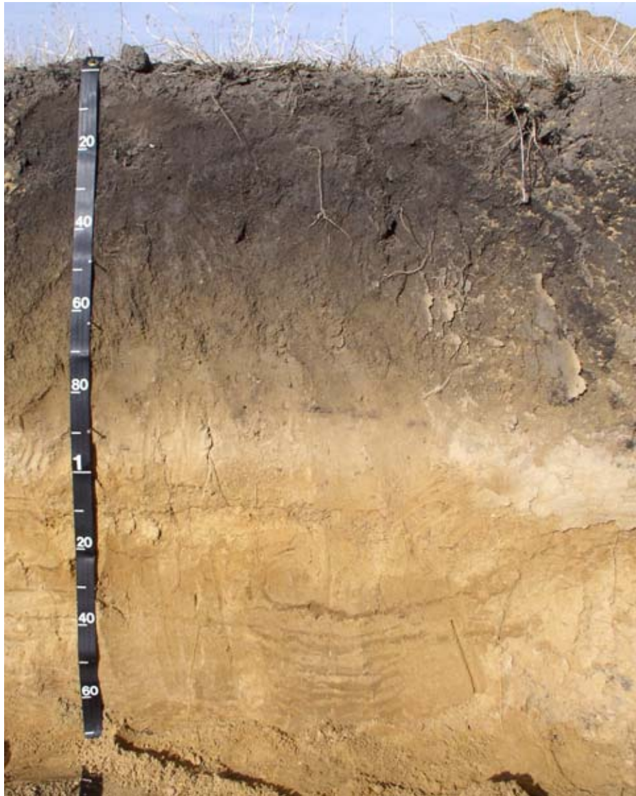
Figure 4.—Profile of a Dickinson soil. These soils are on sandy terraces along the Mississippi River. Depth is marked in centimeters.
