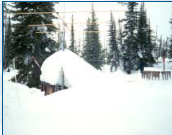
SNOTEL (SNOWpack TELEmetry) sites measure snow water equivalent, precipitation, and temperature. This information allows NRCS hydrologists to forecast stream flows. In 1997, the 16-foot shelter and 16-foot precipitation gage were nearly buried at the Black Bear SNOTEL site in southern Gallatin County.
