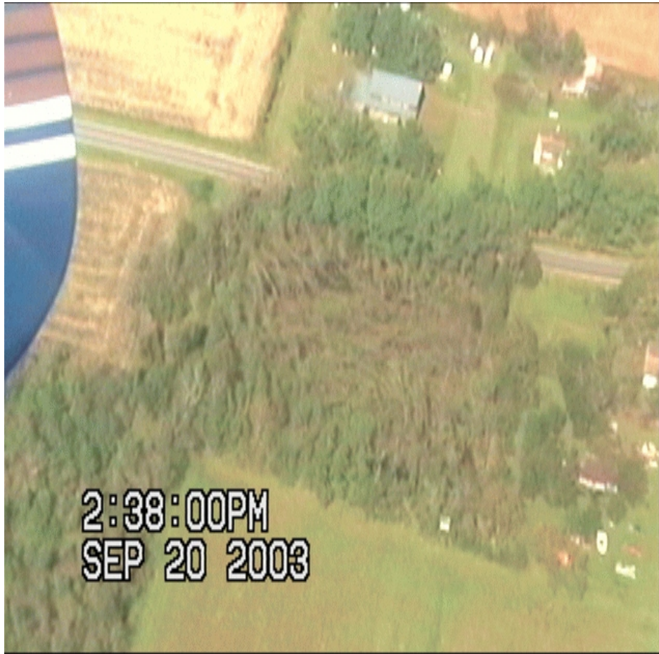
Figure 2 - Video frame of tree damage indicative of a wet microburst.
