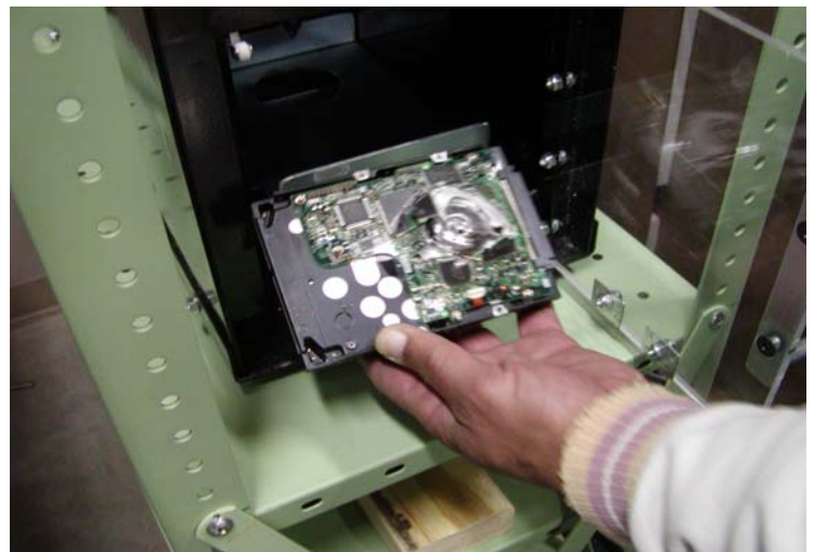
Close up of hard drive after crushing process is completed. Photograph by Kevin Smith
