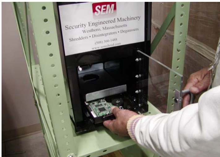
Hard drive being fed into the crusher after being degaussed. Photograph by Kevin Smith
