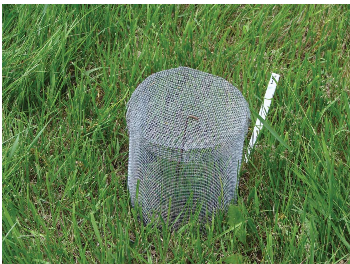
Figure 27 —Cage designed at the Phoenix Lab to allow normal insect thermoregulation.
