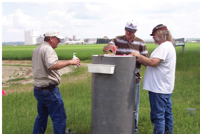
Figure 26 —Field Aerial Application Spray Simulation Tower Technology (FAASSTT) used to apply treatments at the Phoenix Lab.
