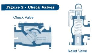
operating principle. Check valves include liftcheck valves, swing-check valves, tilting-disk valves, split-disk valves, and diaphragm-check valves.
