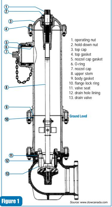
after the hydrant is turned off. As the water drains it creates a vacuum that can be felt at the nozzle. So remember: never tighten the caps until the hydrant finishes draining. And never, ever operate a fire hydrant with any wrench other than the one designed for that particular hydrant.
