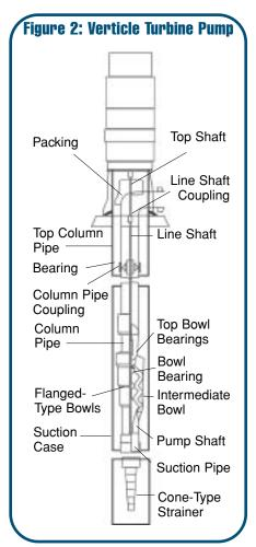
**3.)** They are used mostly for pumping groundwater from wells. The pump is basically a multi-stage centrifugal pump. The impellers of the pump are mounted on a vertical shaft. Each impeller passes water to the next stage through a diffuser shaped so that the water flows vertically to the next diffuser. Each impeller and diffuser is called a stage. The desired output pressure determines the number of stages.
