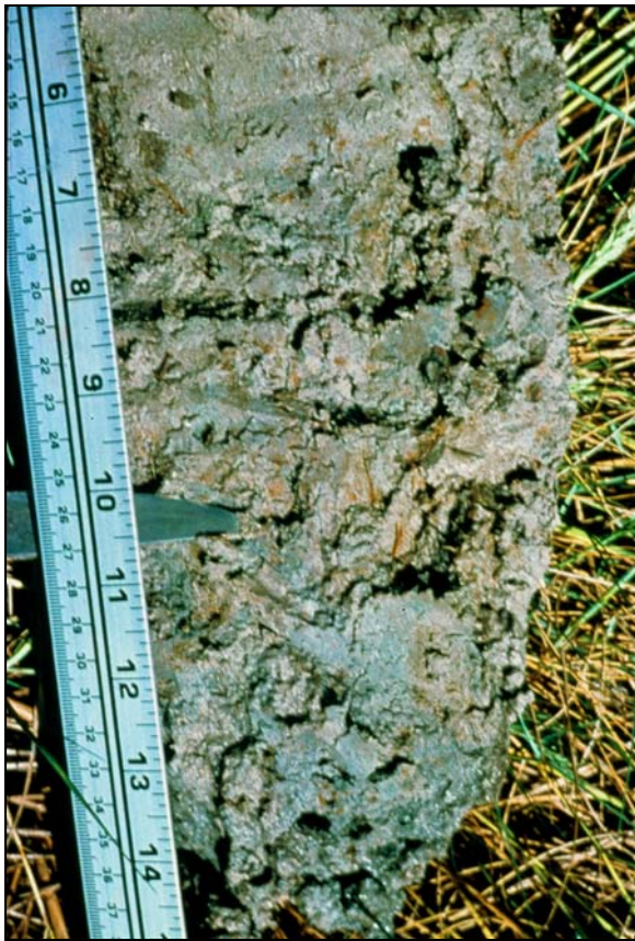
Figure 16. Indicator F3, Depleted Matrix. Redox concentrations are present within a low-chroma matrix.
