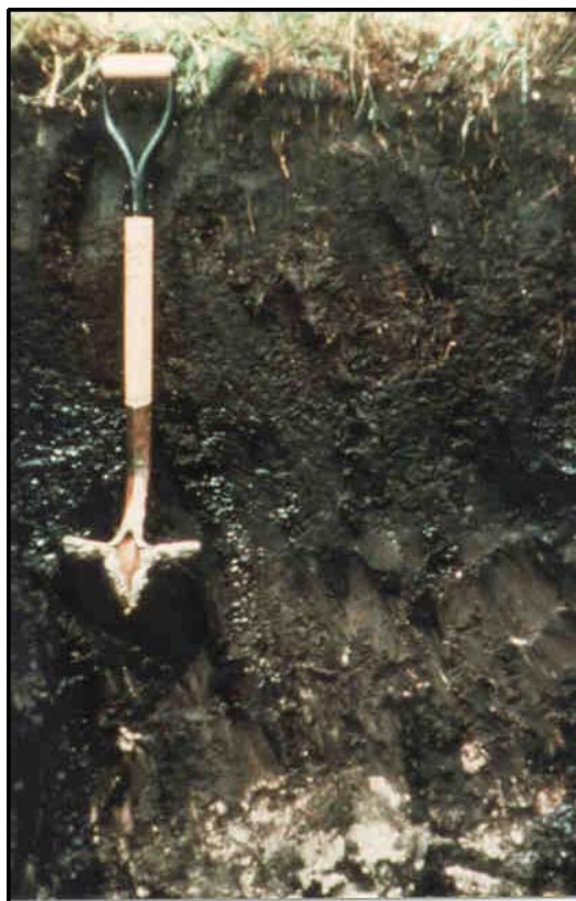
Figure 10. Deep observations may be necessary to identify the depleted or gleyed matrix below the dark surface layer.
