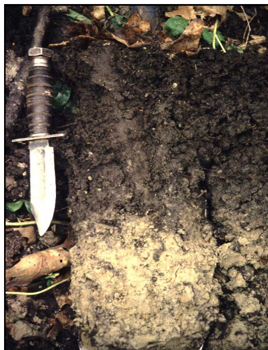
Figure 9. A depleted matrix starts immediately below the black surface layer (approximately 10 in. (25 cm)).
