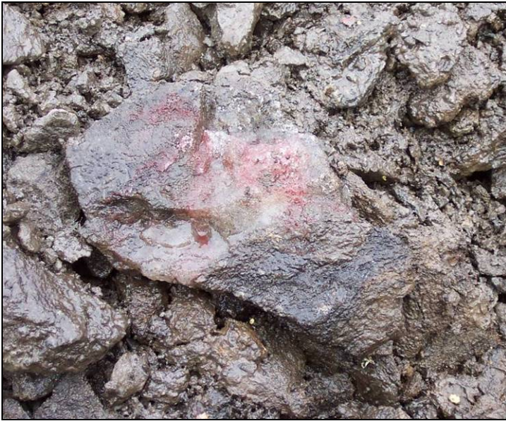
Figure 47. When alpha, alpha-dipyridyl dye is applied to a soil containing reduced iron, a positive reaction is indicated by a pink or red coloration to the treated area.
