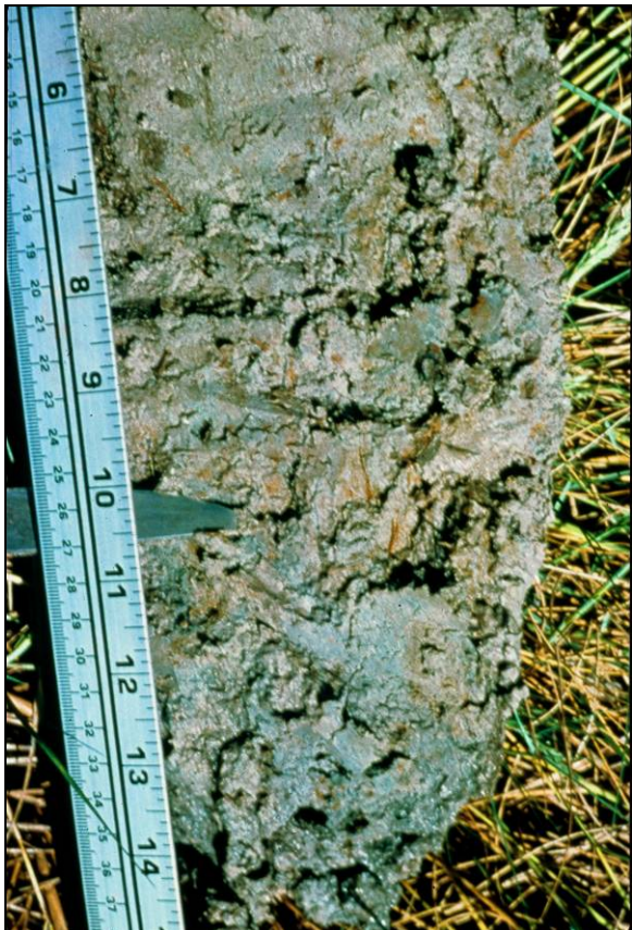
Figure 19. Example of indicator F3 (Depleted Matrix), with redox concentrations present within a low-chroma matrix.
