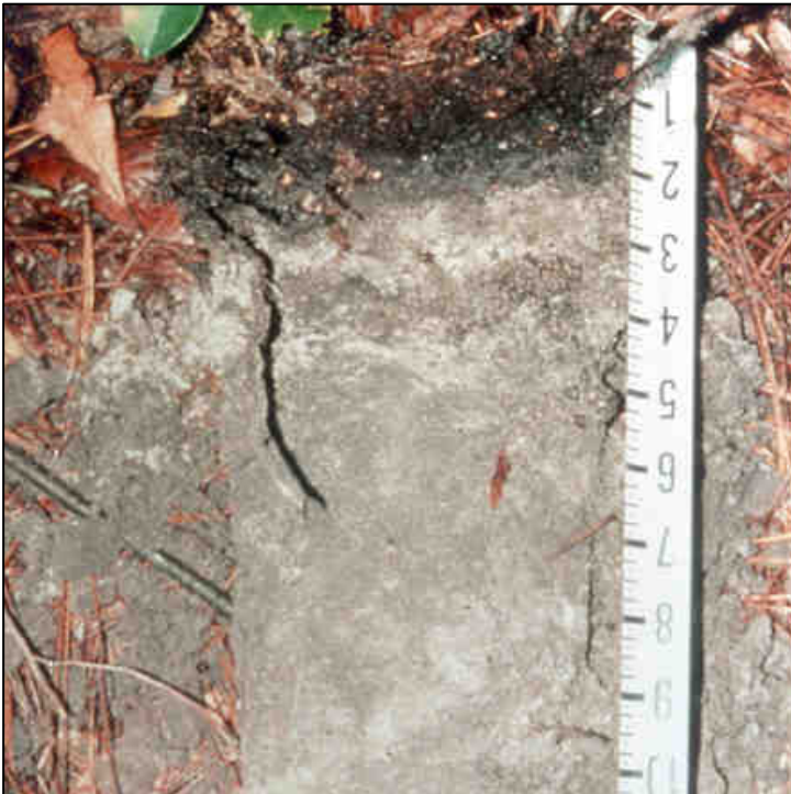
Figure 15. The layer stripped of organic matter begins beneath the dark surface layer (approximately 2 in. (5 cm)).
