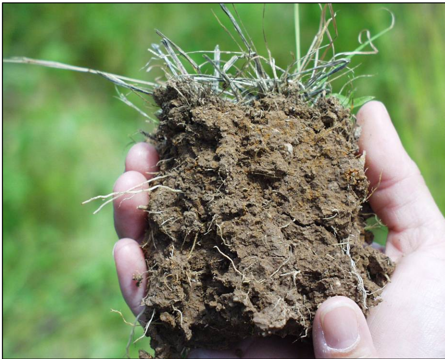
Figure 28. In this example, the layer of redox concentrations begins at the soil surface and is slightly more than 2 in. (5 cm) thick.
