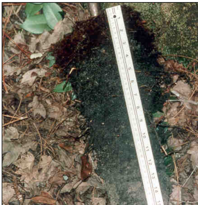
Figure 12. In this example, the muck layer is about 1.5 in. (4 cm) thick and begins at the soil surface. Scale in inches (right) and centimeters (left).
