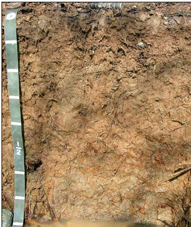
Figure 35. This indicator is restricted to floodplains that are actively receiving sediments. Photo by M. Rabenhorst. Scale in 4-in. (10-cm) increments.
