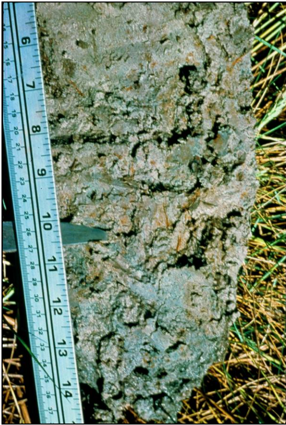
Figure 24. Indicator F3, Depleted Matrix. Redox concentrations are present within a low-chroma matrix.
