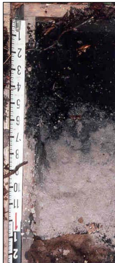
Figure 21. In this soil, the splotchy pattern below the dark surface is due to mobilization and translocation of organic matter. Scale in inches.
