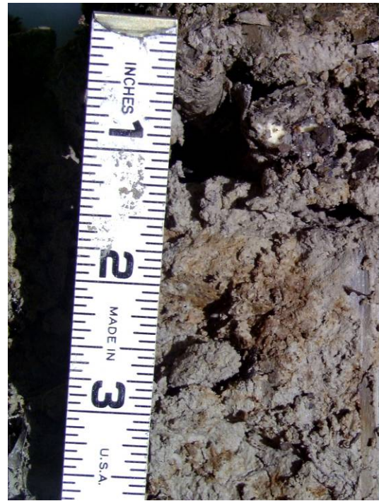
Figure 25. Redox concentrations at 2 in. (5 cm)
