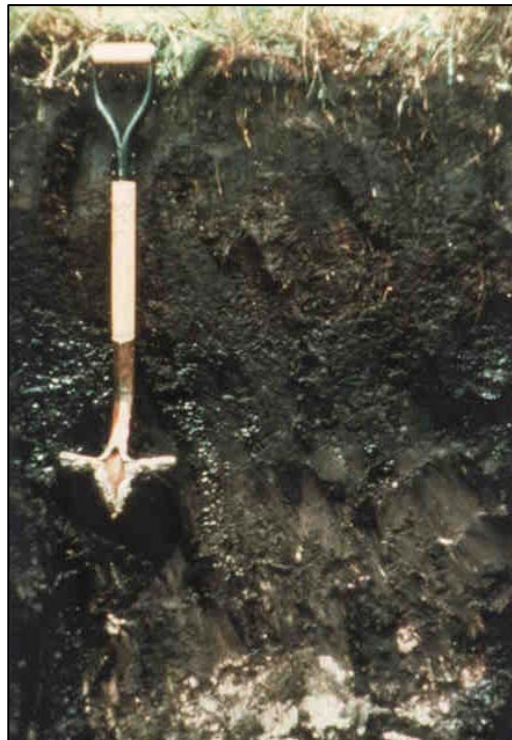
Figure 14. Deep observations may be necessary to identify the depleted or gleyed matrix below the dark surface layer.
