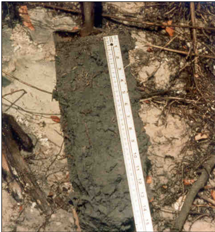
Figure 17. In this example, the gleyed matrix begins at the soil surface.
