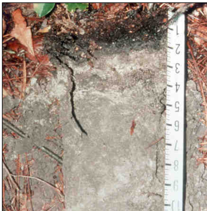
Figure 19. The layer stripped of organic matter begins beneath the dark surface layer (approximately 2 in. (5 cm)).
