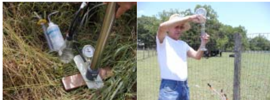
Soil solution sampling procedure: Vacuum at 55-65 kPa is applied to the suction cup lysimeters; and soil solution samples are collected after 18-24 hours
