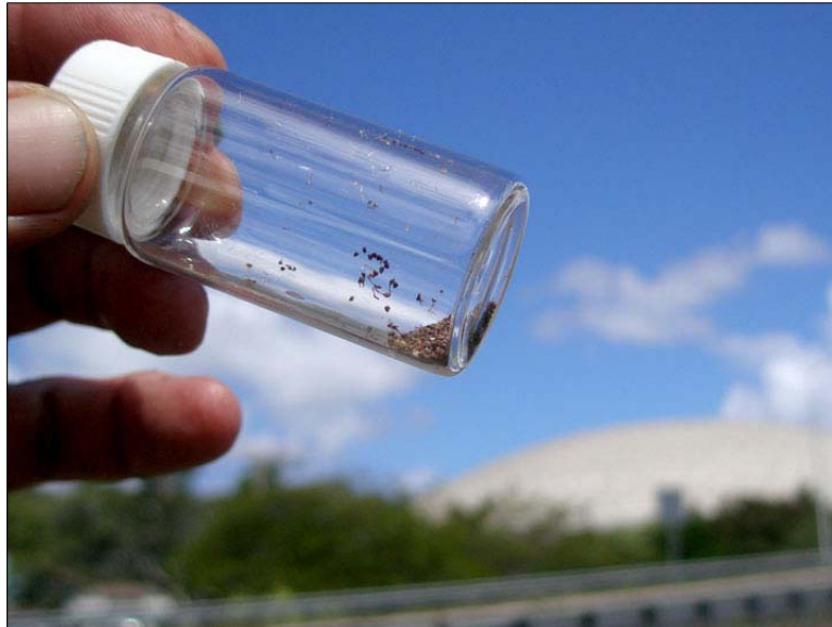
Figure 2. The amount of seed used in the hydroseeding treatment. The vial contains approximately 1490 seeds.
