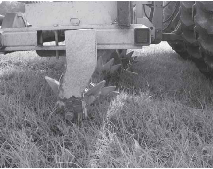
Figure 3. Aeration unit showing tines (knives). Tines are mounted on axles immediately in front of wastewater discharge points.
