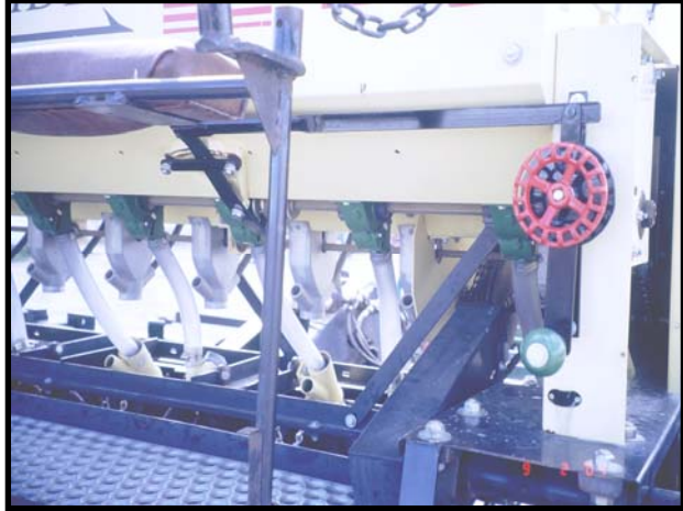
Photo 2.3. Addition of a crank wheel to improve accuracy and ease of calibration.
