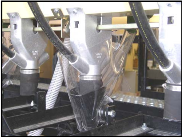
Photo 2.4. Addition of windshields to reduce seed loss during windy conditions.
