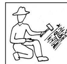
Install stakes perpendicular to mat.
