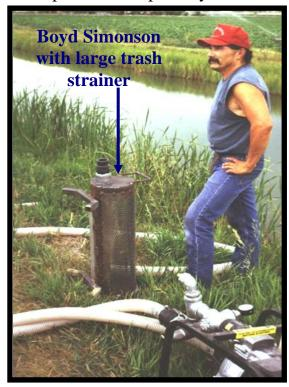
**Note:** Trash Strainer shown was built for large stream systems so it could be perched above the stream bottom and was heavy enough not to move with the stream current. The pump was shipped with a small strainer that attaches to the end of the suction hose for use on smaller stream systems (Not shown).
