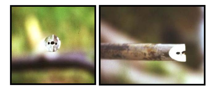
Pictures of the stainless steel nozzles that were welded to ½ in steel pipe. The stainless steel is expected to increase the life of the waterjet. A machinist built the pipe, handle, and nozzles as a single unit. The ball valve is added by the end user.
