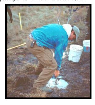
As the user pulls the waterjet back up out of the hole, the nozzle should be rotated back and forth to increase the size of the hole. The rotation should continue the entire length of the hole from the bottom to the ground surface. The waterjet probe is ½ in diameter and the user should be
