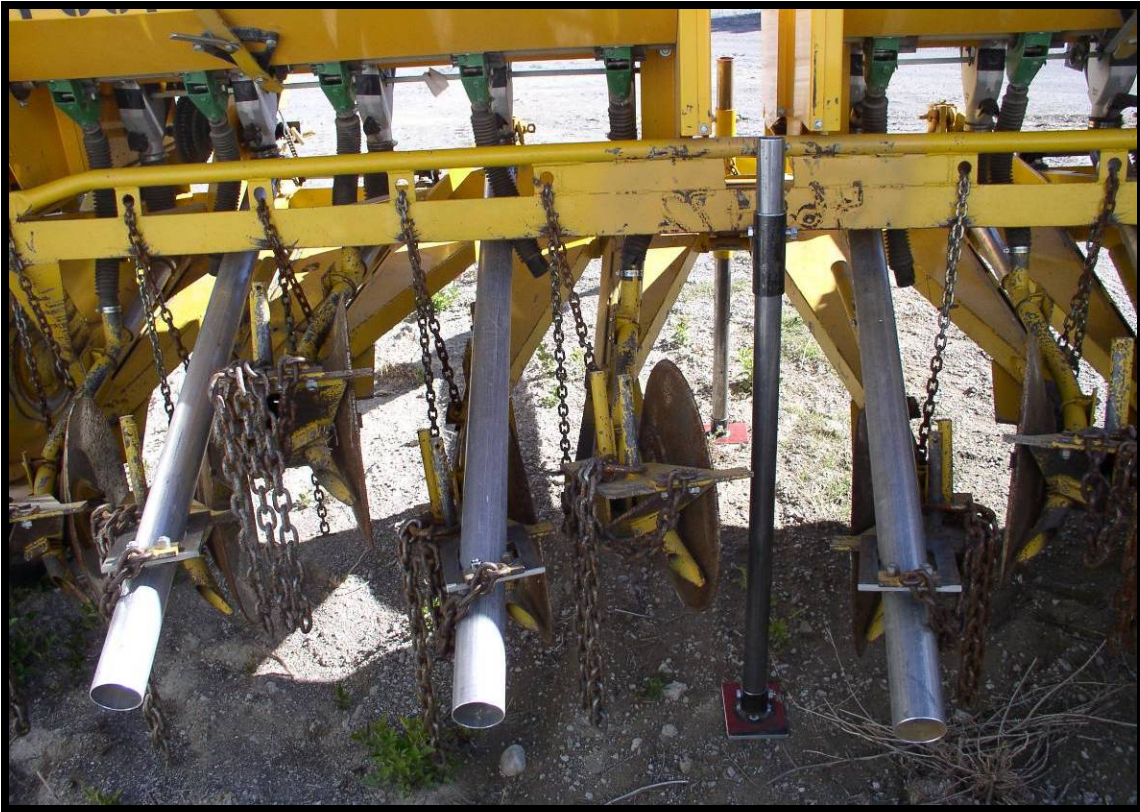
Kemmerer drill with modified drop tubes and jack stands for safety.
