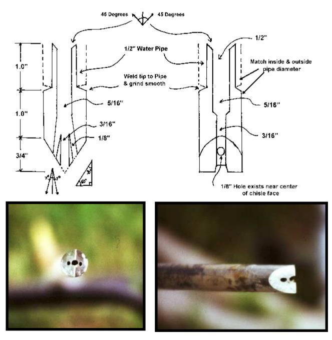
Pictures of the stainless steel nozzles that were welded to  $\frac{1}{2}$  in steel pipe. The stainless steel is expected to increase the life of the waterjet. A machinist built the pipe, handle, and nozzles as a single unit. The ball valve is added by the end user.
