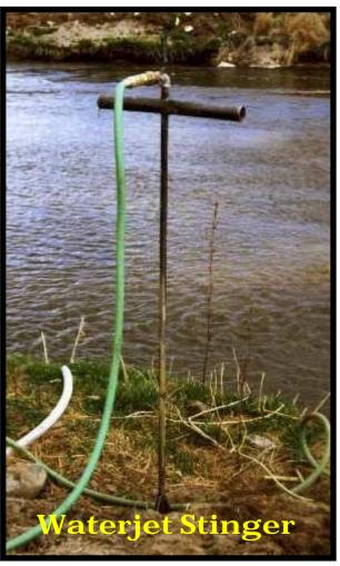
and Ogle 1994). Most riparian and stream protection projects require planting depths of 3-6 ft. The biggest problem we faced was finding a method and developing equipment that could dig a hole more than 3-4 ft deep quickly and efficiently. The Waterjet Stinger is the result of this equipment development effort.
