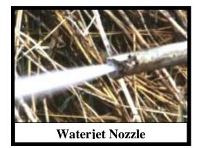
Simonson, PMC Biological Technician, used the paper written by Drake and Langel (1998) and attempted to modify their design to better fit the coarse soils in the Intermountain West. He started with the actual probe itself. A local machinist used the detailed drawing to build the nozzle out of stainless steel and welded it to a ½ in steel pipe. Boyd added a T-handle at the top to help with the planting operation and a ball valve at the handle to turn the water on and off (see Appendix A).
