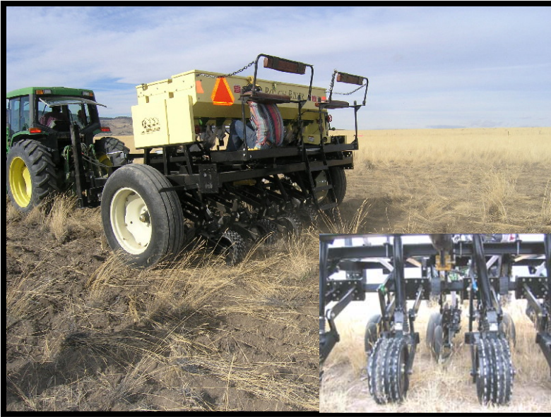
The Truax Roughrider Range drill (above) being used to seed test plots in Utah. Addition of broadcast seeders (inset) allows planting shallow-seeded species in alternating rows with deep-seeded species in a single operation.
