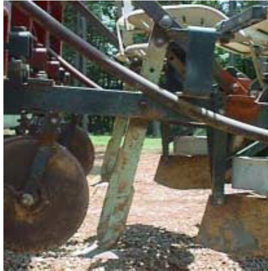
Fig. 1. Shank with 6 inch sweep added for planting in high residue.
