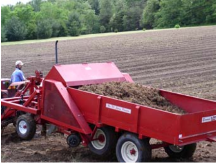
Plant Materials Center's No-till Bermudagrass Sprig Planter
