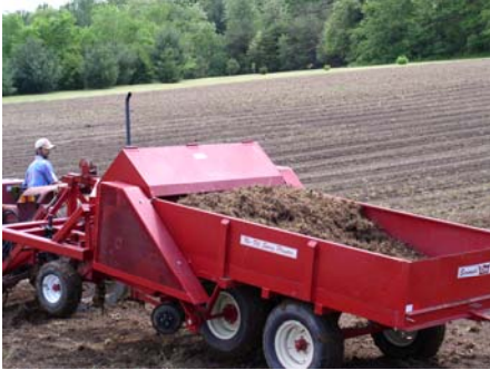
Plant Materials Center's No-till Bermudagrass Sprig Planter
