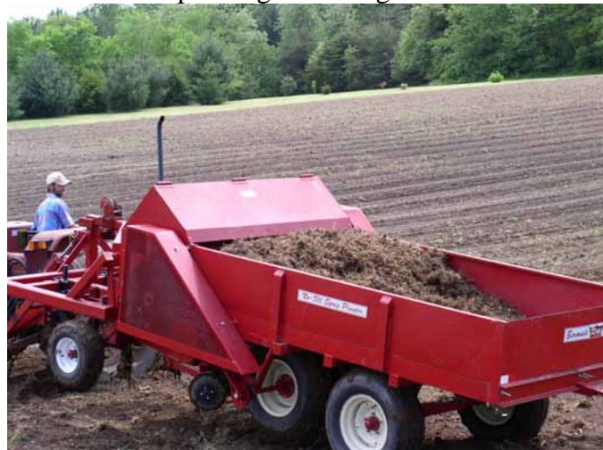
Plant Materials Center’s No-till Bermudagrass Sprig Planter
