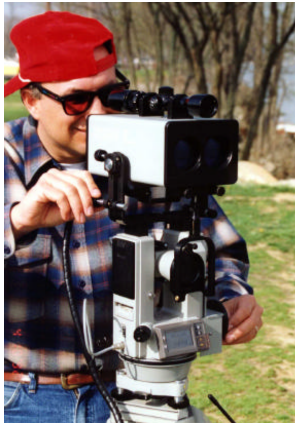
Figure 27. Two-piece range-azimuth system used for detailed data collection.
