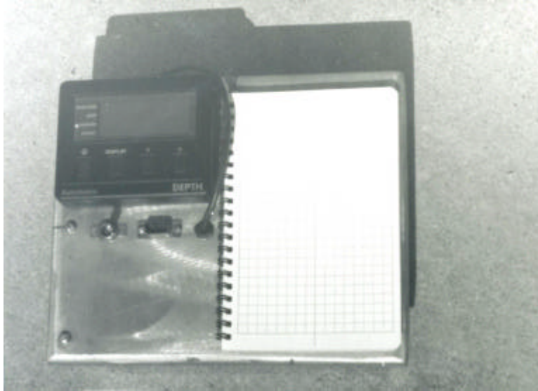
Figure 23. Numerical-display echo sounder mounted in box with batteries and area for notepad.
