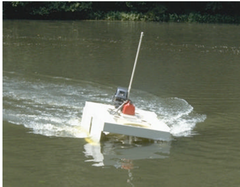
Figure 36. Instability of swath boat during testing.
