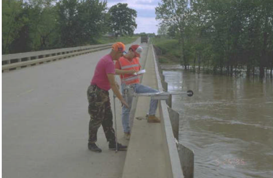
Figure 18. Bridge board with standard stream-gaging equipment.
