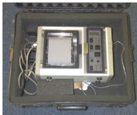
Figure 30. Waterproof case with digital echo sounder used for detailed data collection.
