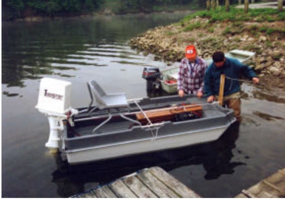
Figure 39. Polyethylene twin-hull boat tested for use as a remote-control boat.
