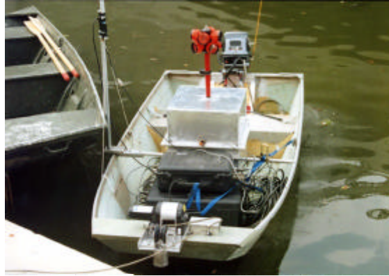
Figure 40. Flat-bottom jon boat modified for use as a remote-control boat.
