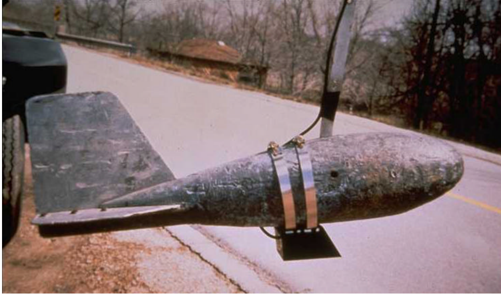
Figure 19. Closeup of transducer mounted to the bottom of a Columbus weight.
