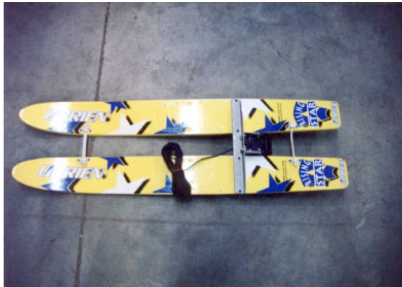
Figure 26. Water skis modified to deploy a transducer
