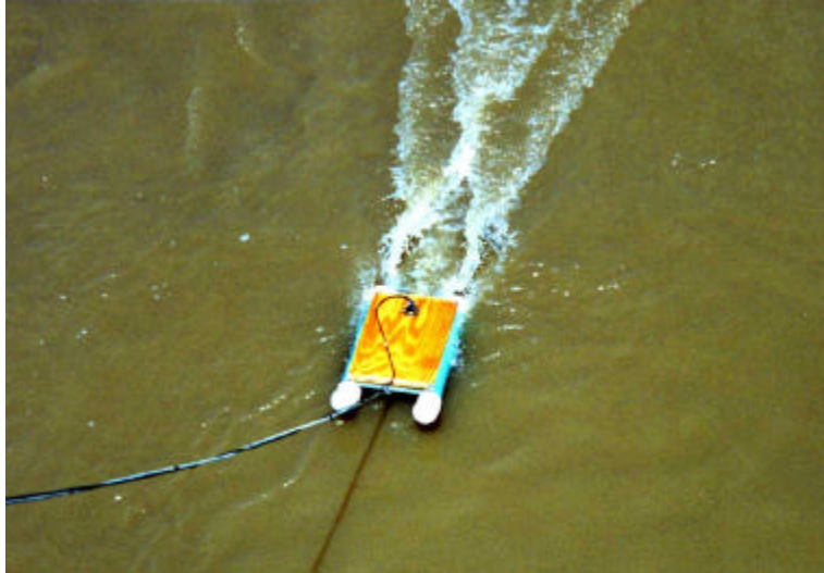
Figure 25. PVC-pontoon float for deploying a transducer.
