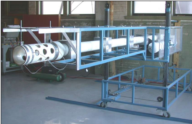
Forest Products Laboratory's air-pressurized Debris Launcher.
