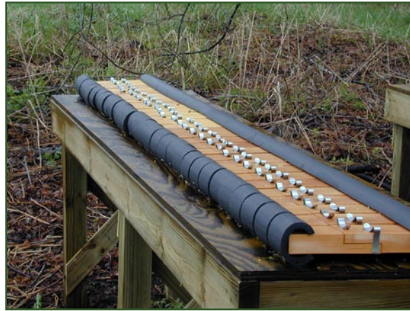
Aboveground L-joint test.
