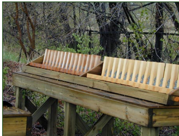
Aboveground L-joint test.
