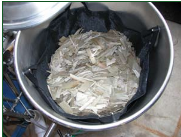
CCA-treated wood flakes prior to pilot-scale remediation.
