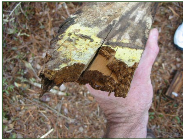
Copper-tolerant brown-rot fungus on preservative-treated specimen.
